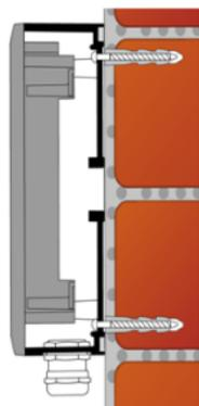
The 2N<sup>®</sup> Helios IP Uni AI box, (Part No. **9153003**) is designed for wall mounting especially where flush mounting is impossible such as on carrier elements of industrial objects.
