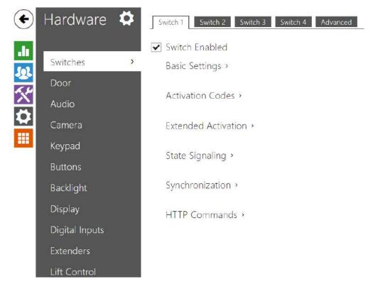
Switches provide a very flexible and efficient control of such intercom peripherals as electric door locks, lighting, additional ringing signalling, and so on. **2N IP intercoms** allows you to configure up to 4 (depending on model types) independent all-purpose switches.
