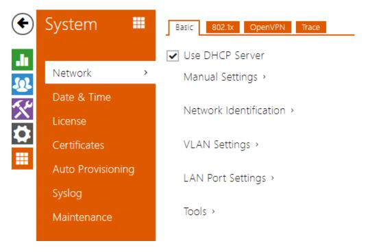
As the **2N IP intercom** is connected to the LAN, make sure that its IP address has been set correctly or obtained from the LAN DHCP server. Configure the IP address and DHCP in the **Network** subsection.
