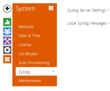
The **2N IP intercoms** allow you to send system messages to the Syslog server including relevant information on the device states and processes for recording, analysis and audit. It is unnecessary to configure this service for common intercom operation.
