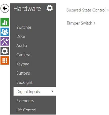
In this configuration section set the parameters associated with digital inputs and their interconnections with other intercom functions. The digital inputs are available in
