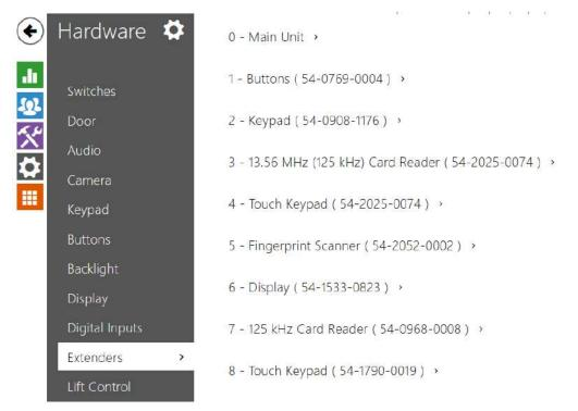
The **2N<sup>®</sup> IP Verso** intercoms can be enhanced with extending modules connected to the intercom basic unit. The following modules are available:
