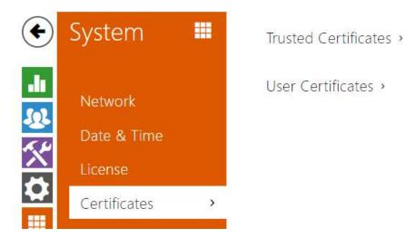
Some **2N IP intercom** network services use the Transaction Layer Security (TLS) protocol for communication with other LAN devices to prevent third parties from monitoring and/or modifying the communication contents. Unilateral or bilateral authentication based on certificates and private keys is needed for establishing connections via TLS.
