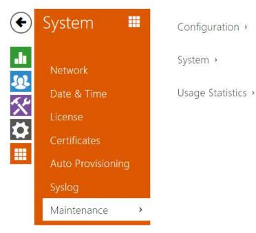
Use this menu to maintain your intercom configuration and firmware. You can back up and reset all parameters, update firmware and/or reset default settings here.
