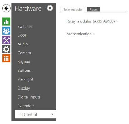
To control the floor lift access, connect the AXIS A9188 relay module to the 2N IP intercom (**2N**<sup>®</sup> **IP Verso**, **2N**<sup>®</sup> **IP Force**, **2N**<sup>®</sup> **IP Safety**, **2N**<sup>®</sup> **IP Vario**). Up to 8 relay modules can be connected to one 2N IP intercom, each of which can control up to 8 floors, which makes a total of 64. Make sure that the IP intercoms Lift module license is active (Part No. 9137916) to make this function work.
