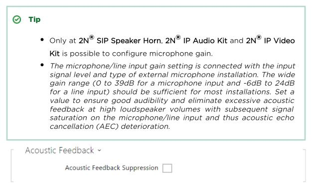
• Acoustic feedback filter - set automatic suppression of acoustic feedback (typically whistling) between the intercom speaker and phone handset if located in close proximity to the intercom. This mode is disabled by default.
