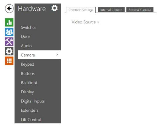
This menu is only available in the **2N IP intercom** models that are equipped with an internal camera or can be connected to an external camera. The camera signal can be streamed directly into the call via a videophone, sent by E-mail, streamed via ONVIF /RTSP to another device (a video surveillance device, e.g.), or simply HTTP downloaded from the intercom in the JPEG format.
