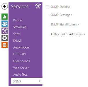
The **2N IP intercoms** integrate a remote intercom supervision functionality via the SNMP. The integrated SNMP agent becomes available when the **Enhanced Integration** license key is added. The intercoms support the SNMP version 2c.
