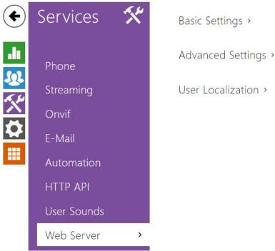
Veb Server > You can configure your 2N IP intercom using a standard browser which accesses the integrated web server. Use the secured HTTPS protocol for communication between the browser and intercom. Having accessed the intercom, enter the login name and password. The default login name and password are admin and 2n respectively. We recommend you to change the default password as soon as possible.
