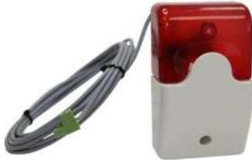
Required for light and sound alarms. Has 1.5m length. Connected to the electronic relay 12V DC, 0.25A to monitoring systems.
