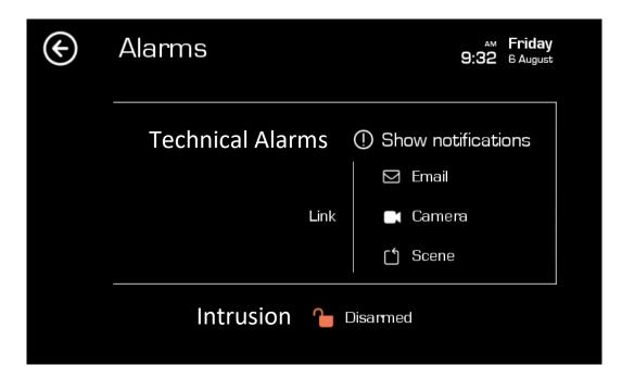
Every time a technical alarm is activated in the installation, a warning icon will be displayed next to the Wi-Fi signal icon. If you want to know what the alarm refers to, you must click on the warning icon (which will blink during the warning) or on the alarms menu to display the notifications.
