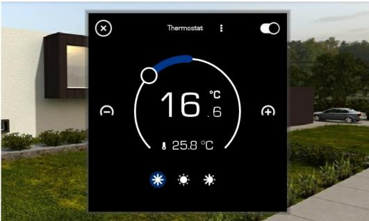
If the thermostat is off, all configurable thermostat options remain disabled. It would also be impossible to change the set temperature. If you want to activate the thermostat you have to put it in the ON position.
